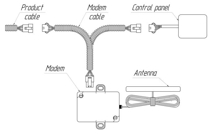
Fig. 3. Modem connection to AUTOTERM heaters
