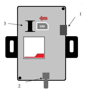
Fig. 2. To insert SIM card
